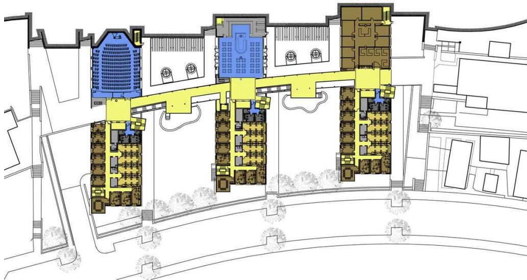
Diagram of 3rd floor of Rothberg Building. This is the entrance level from the west (top of diagram). Auditorium (left) and cafeteria (center) are marked in blue. The south (left) and central wings will be initially occupied. The shell of the north wing (right) is completed, and is kept for future expansion.
